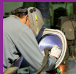
Welding stainless steel sanitary fittings DELABIE's factory in Aveiro, Portugal
