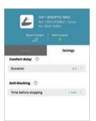
The comfort timing (tap shut-off delay once hands or body are removed from in front the infrared sensor) can also be adjusted.
